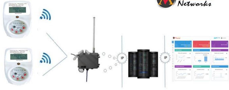
LoRa(LoRAWAN) Smart Gateway LoRa(LoRAWAN) Application Server
